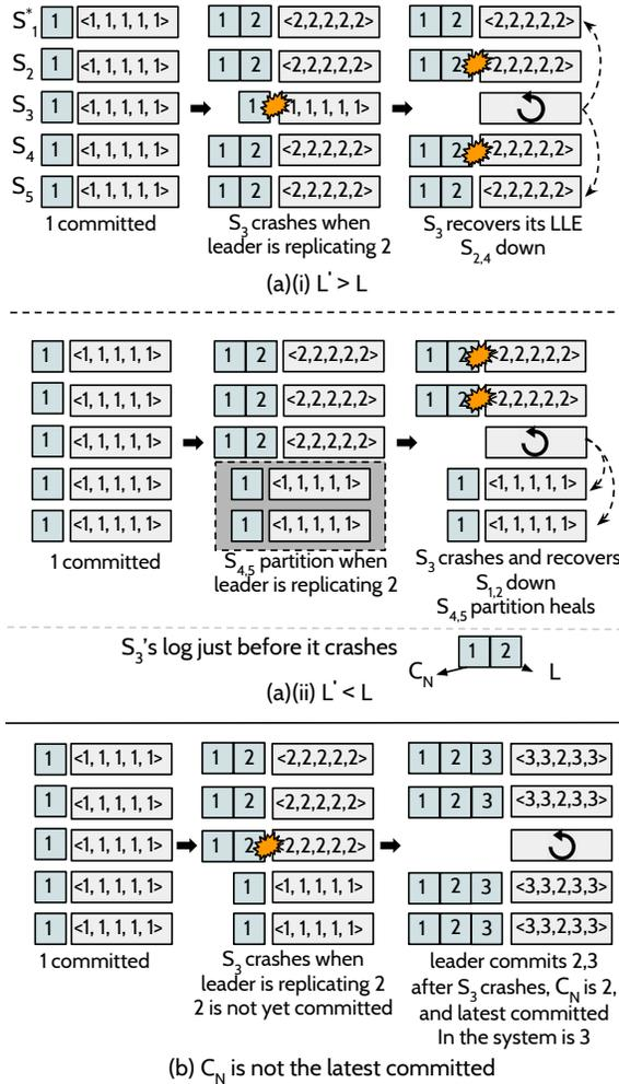
Figure 4: **LLE Recovery.** The figure shows how  $L'$  may not be equal to  $L$ . For each node, we show its log and  $LLE-MAP_S$ . The leader ( $S_1$ ) is marked \*; crashed nodes are annotated with a crash symbol; nodes partitioned are shown in a dotted box; epochs are not shown.
