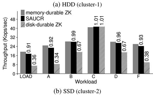
Figure 8: **Macro-benchmarks.** The figures show the throughput under various YCSB workloads for memory-durable ZK, SAUCR, and disk-durable ZK for eight clients. The number on top of each bar shows the performance normalized to that of memory-durable ZK.
