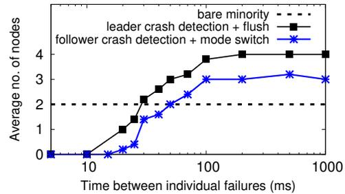
Figure 11: **Correlated Failure Reaction.** The figure shows how quickly SAUCR reacts to correlated failures; the y-axis denotes the number of nodes that detect and flush to disk before all nodes crash when we vary the time between the individual failures (x-axis). We conduct this experiment on SSDs.
